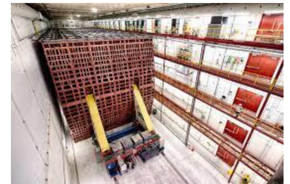
NOvA Far Detector, consists of liquid scintillator covered in PVC pipes (Picture from Fermilab)
