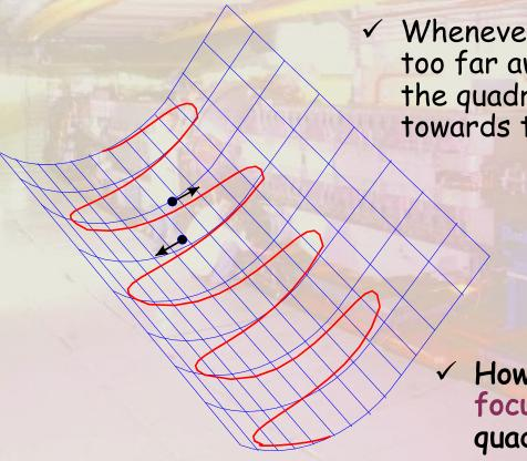
✓ Whenever a particle beam diverges too far away from the central orbit the quadrupoles focus them back towards the central orbit.
