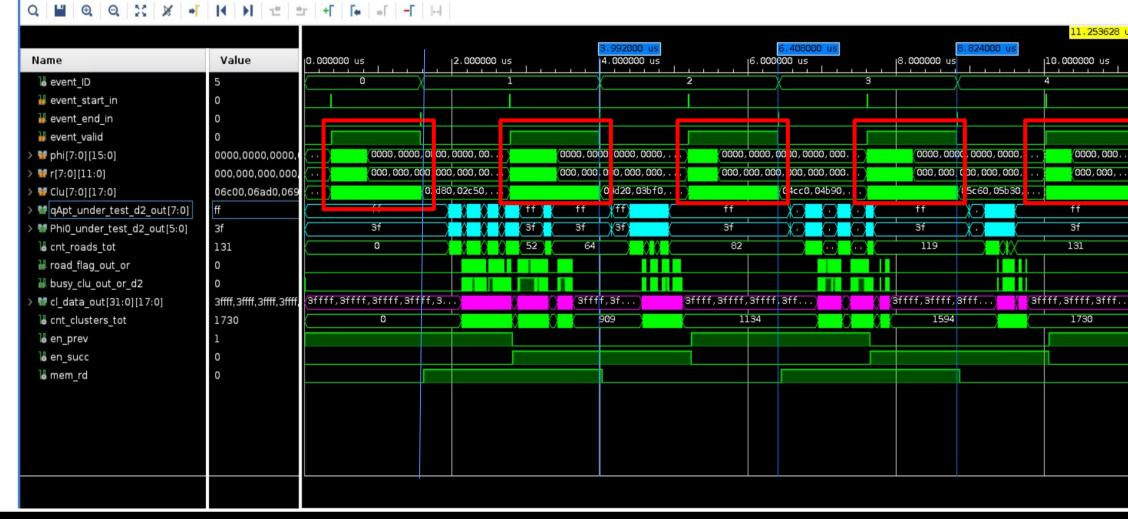
The design has been featured with a double storage structure for all the necessary information, including a second accumulator and a second store for the event clusters. This allows to process two events concurrently and consider the firmware as two macro-blocks working separately. The left image shows a simulation where the output stream of the firmware for an event is active, while the input of the next event has been acquired.
