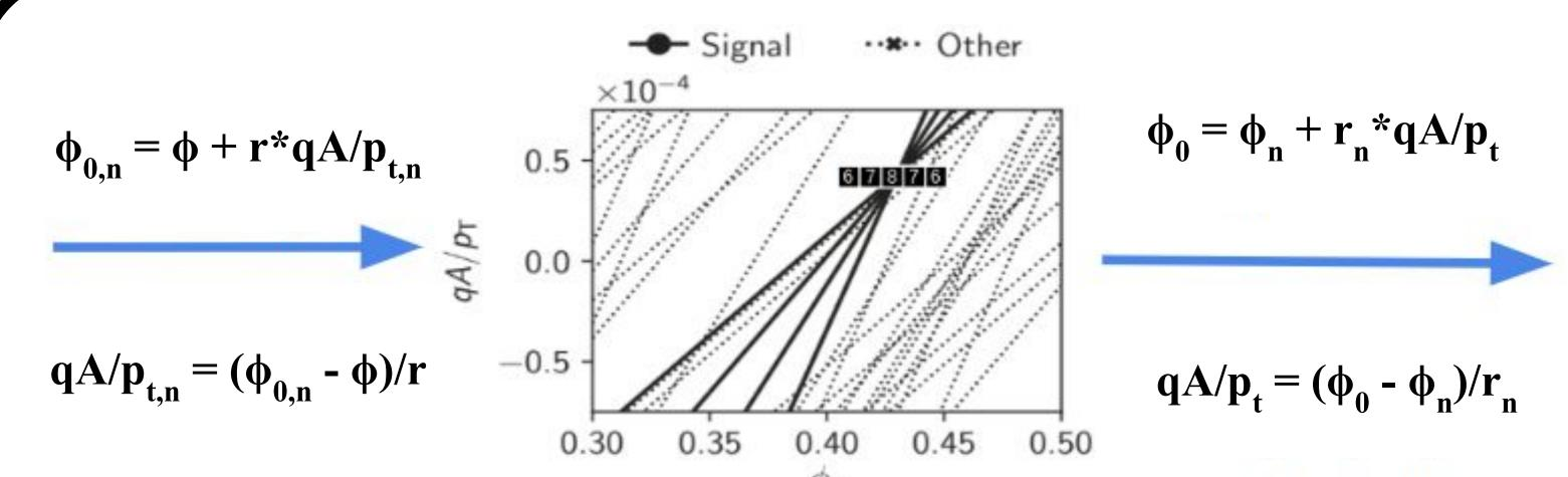
A qA/ $p_t$ : $\phi_0$  2D histogram called "Accumulator" (center of the image on the left), made of several bins, is the core of the algorithm. The HT operations are:
