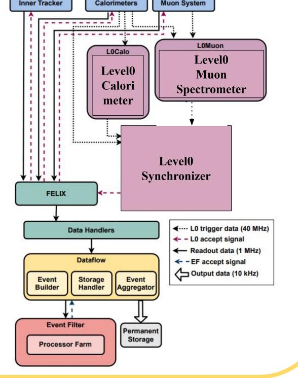
EVENT FILTER TRACKING The Event Filter Tracking is an ATLAS project aimed to implement a technologically commodity hardware architecture to join the EF, exploring and exploiting FPGAs, GPUs and high-performing CPUs. It is studying the performance of the Hough Transform (HT) tracking algorithm to use at Trigger level. To exploit it, the ATLAS coordinate system is in polar coordinates, with the position of the particle be defined as radius "r" and azimuth angle " $\phi$ ".
