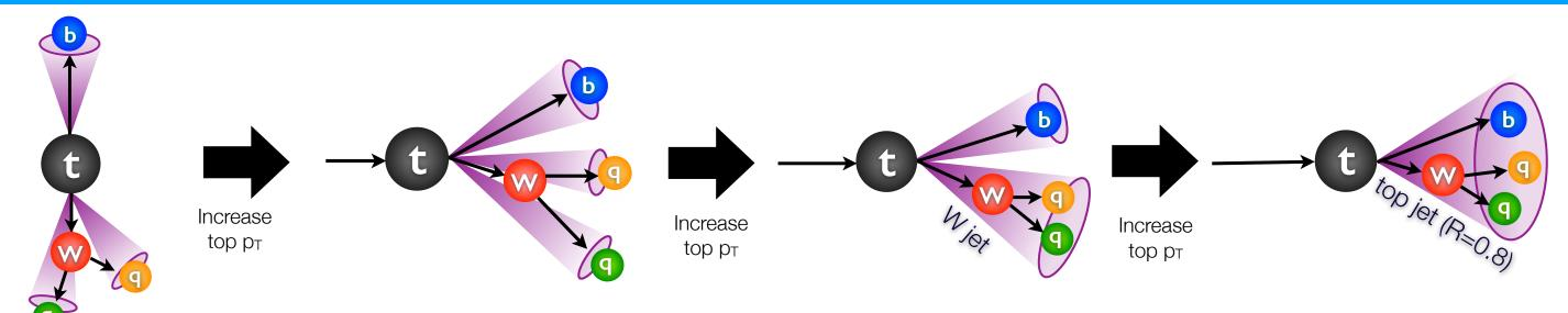
A schematic showing the way in which the subjets of a top quark decay merge with increasing  $p_T$
