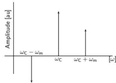
$$V_{AM}(t) = A_C \cos(\omega_C t) + \frac{\alpha A_C}{2} [\cos((\omega_C + \omega_m)t) + \cos((\omega_C - \omega_m)t)]$$
