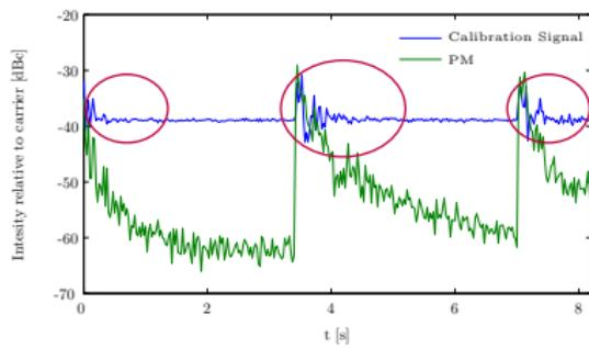
Data taken with 25 ns beam of 4 batches at SPS flat bottom
