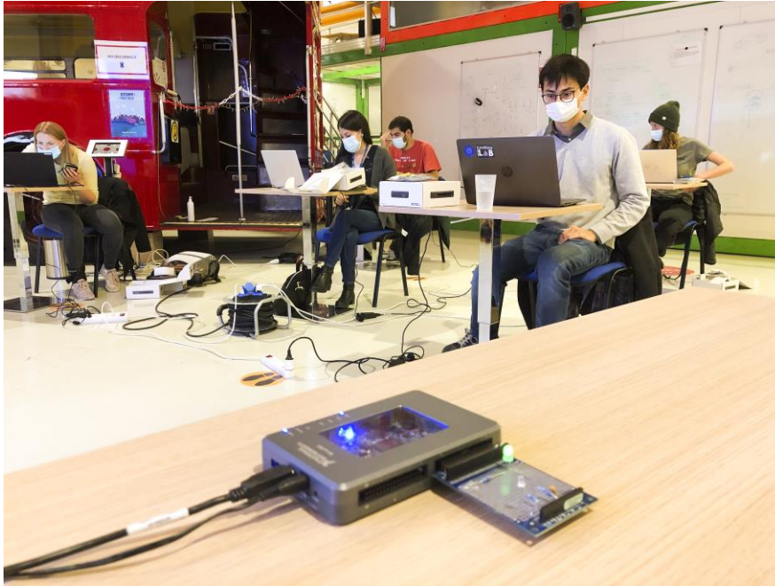
Programming an FPGA inside a myRIO
