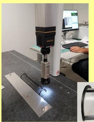
b) The second set of measurements. Coordinate measurements were done by Mitutoyo machine in the same five cradle points - cradle <u>with</u> <u>Aerospace Fiberglass as an</u> <u>emulator of silicon layer</u>
