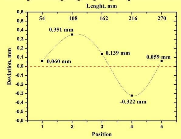
One can see that after the Aerospace Fiberglass plate gluing <u>the distance between the</u> <u>cradle longerons has changed: it is increased by 60 um in the region of the end of the</u> <u>cradle (i.e. near semi-rings)</u>. Maximal deviation was about 351 um in the region of the cradle centre.
