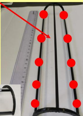
**Investigations of the properties of carbon fiber cradle with new extra-thin carbon fiber longerons and aerospace fiberglass as emulator silicon layer.** On this picture the mean deviation between initial (without Aerospace Fiberglass) and final (after the Aerospace Fiberglass gluing) stages is plotted.
