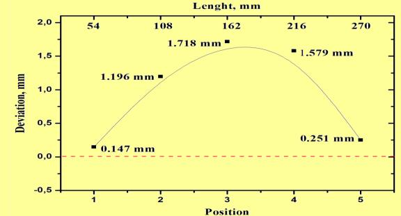
➤ Conclusion №1 with extra-thin longerons: one can need more thick longerons and semirings in case of the given radius (30mm) of bent Si-sensor.
