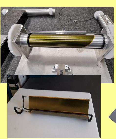
Again two sets of the measurements by using Mitutoyo machine without silicon dummy sheet and after the Si dummy sheet gluing were carried out.
