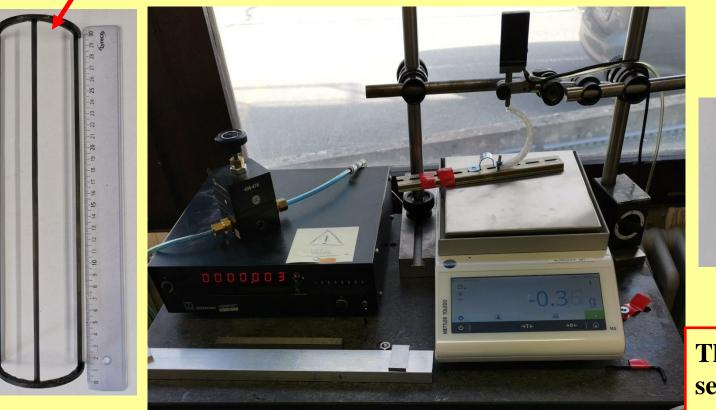
The sagging measurements of carbon fiber semi-ring done at CERN (at Piter's lab.)
