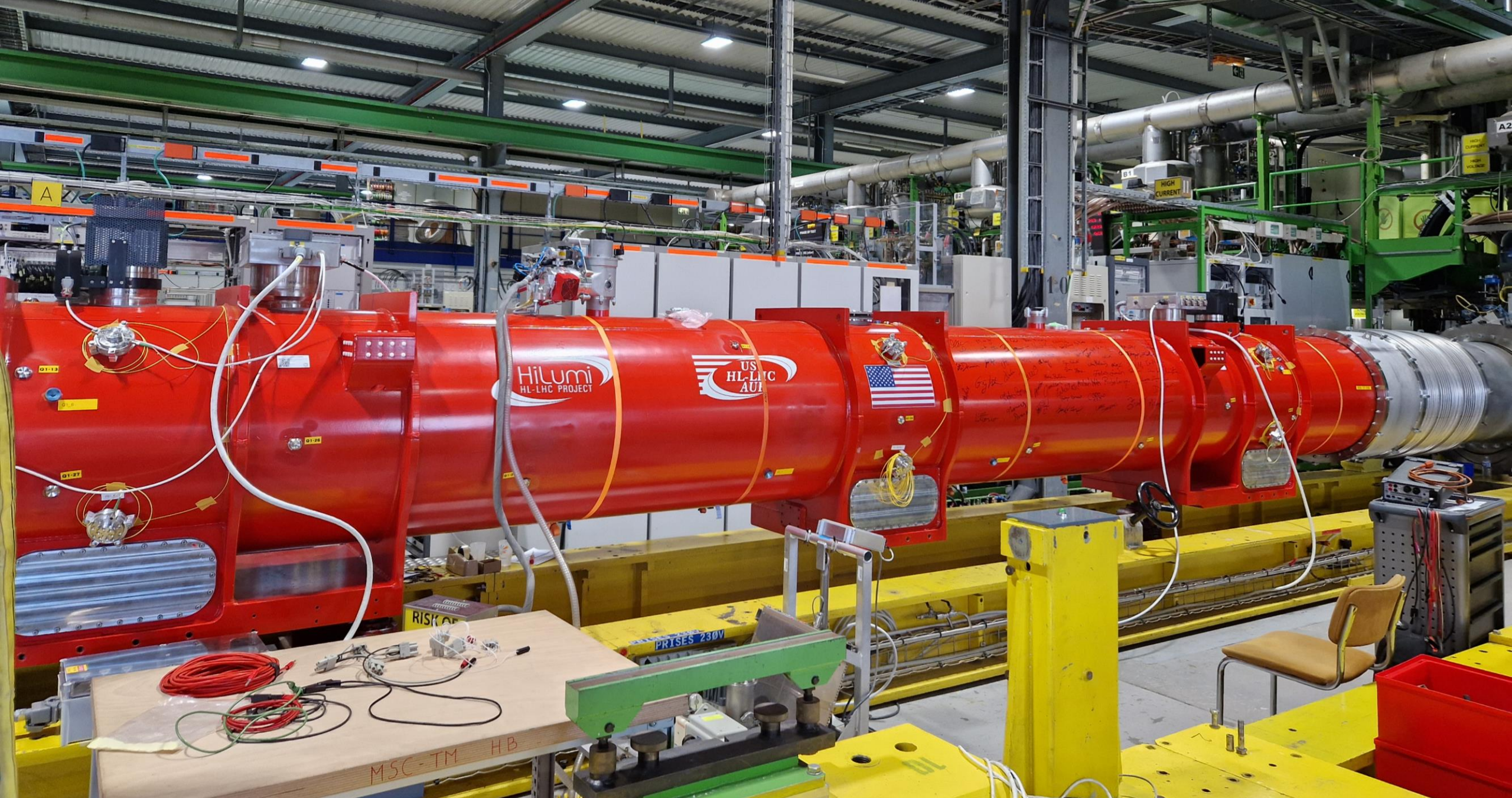
LQXFA01 AKA Q1/Q3 – FIRST QUADRUPOLE CRYO-ASSEMBLY PRODUCED IN THE US BEING TESTED IN SM18
