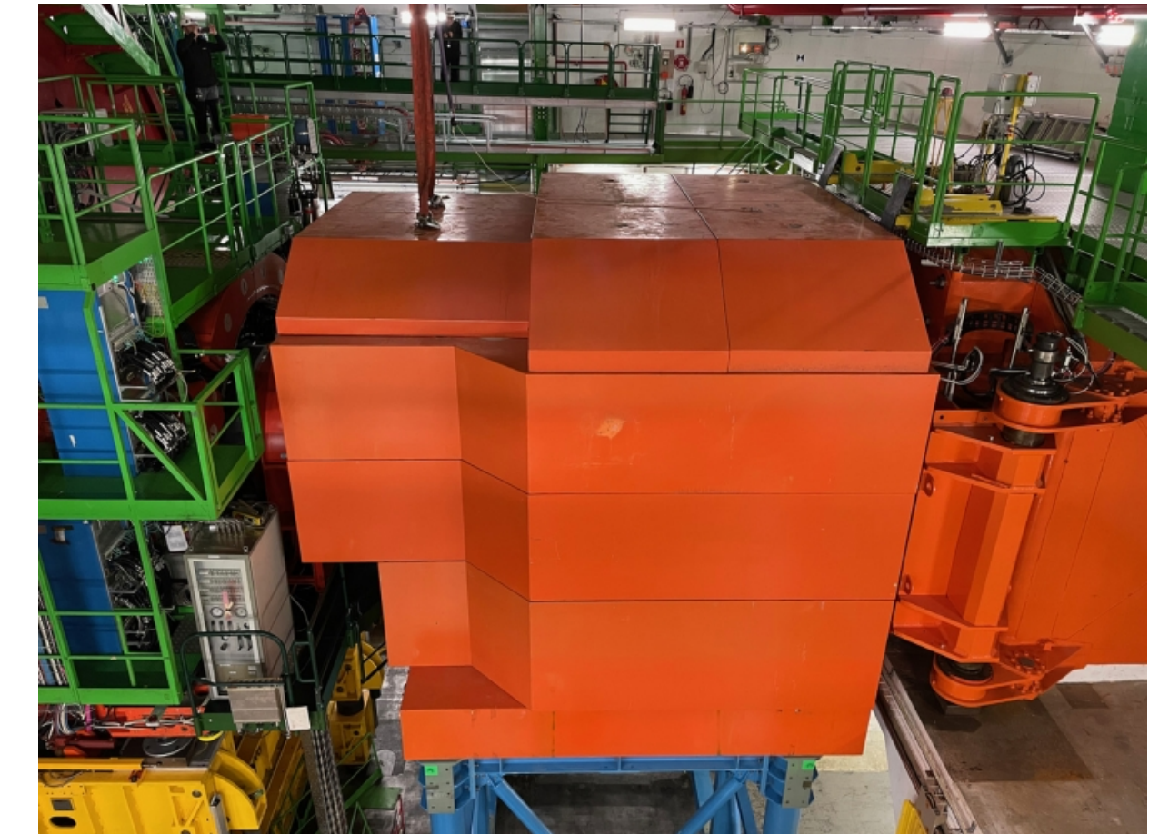
First new shielding for reduced background ( Phase 2 version )
