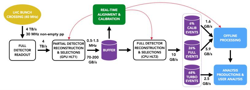
Hardware-based L0 would not allow profiting from higher luminosity → full detector readout (4 TB/s) + 2 levels of software-based trigger
