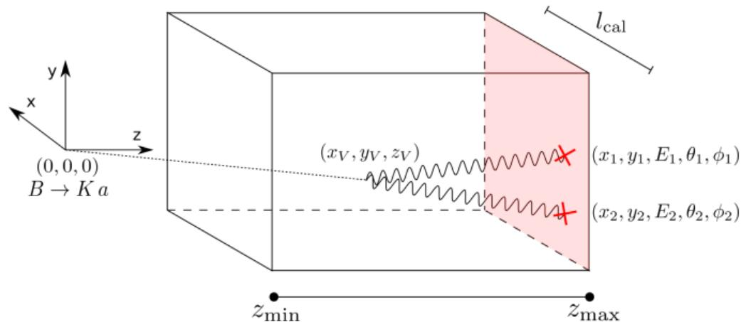
Geometry of the detector:  $z_{\text{min}} = 10\text{m}$ ,  $z_{\text{max}} = 35\text{m}$ ,  $l_{\text{cal}} = 2.5\text{m}$
