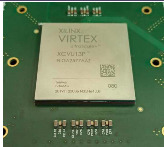
XCVU13P FPGA mounted on the BMTL-1 ATCA board
