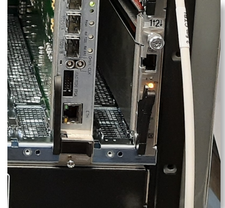
Extraction handles with hot swap switch
