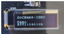
Figure 28: SoCMake-Ibex booting on FPGA
