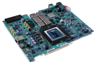
VPK120 Essential Hard IP Development Kit (VP1202 Silicon)
