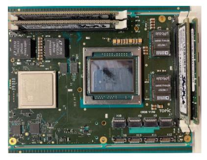
~150W max. total power consumption 0.85V/120A core supply Liquid cooling solution Must support full device utilization
