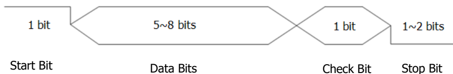
Figure 5-13 Schematic Diagram of RS232 Protocol
