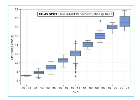
In the plot: CPU time per event during a 2022 data-taking run, as a function of  $\langle \mu \rangle$ . The boxes indicate the coverage of the middle two quartiles of data, with a line at the median. The whiskers indicate the location of the data point furthest from the median, within 1.5 times the difference between the 3rd and 1st quartiles (the <u>IQR</u>). The points indicate outliers.
