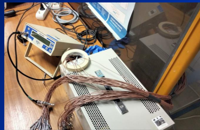
Single channel electrometer used as charge integrator
