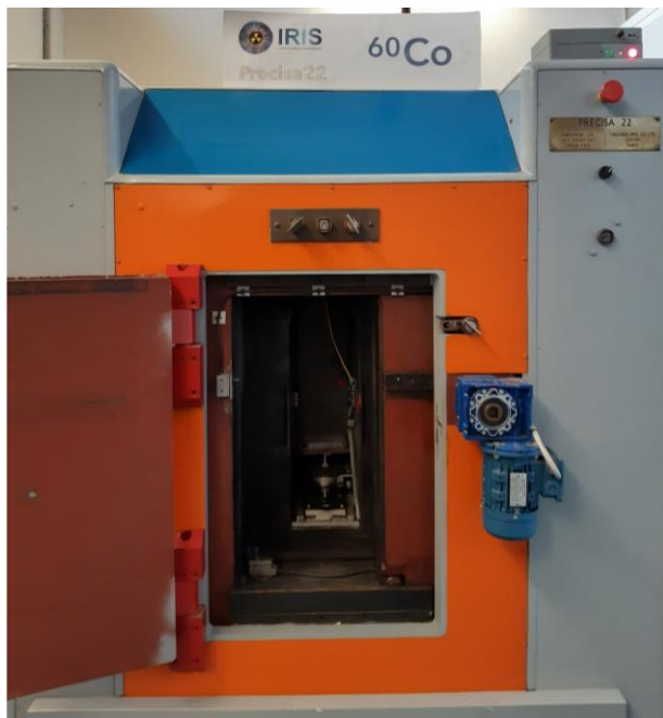
PRECISA22 - ^{60}\text{Co} irradiator used in the first experiments.
