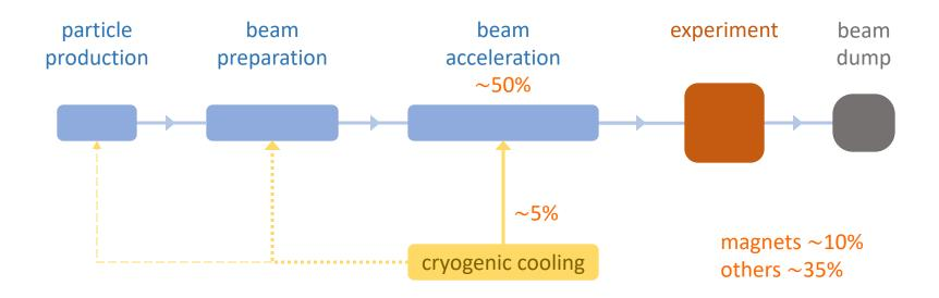
Typical power consumption for an electron-positron Higgs Factory the highest priority next collider for particle physics
