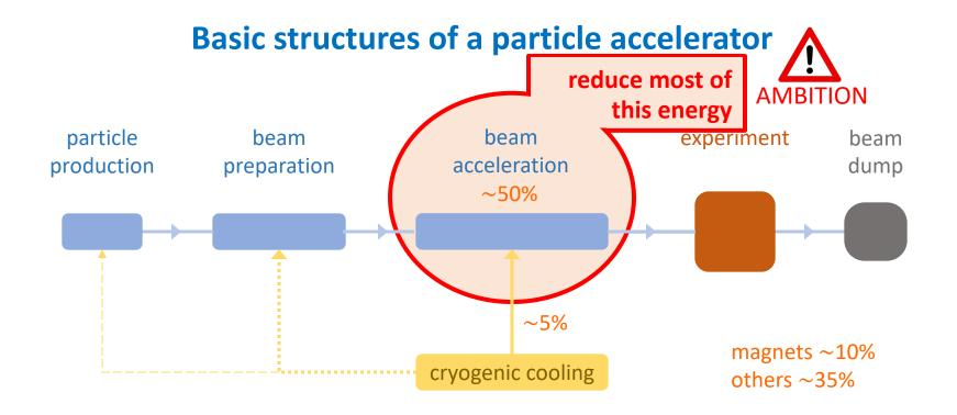
Typical power consumption for an electron-positron Higgs Factory the highest priority next collider for particle physics
