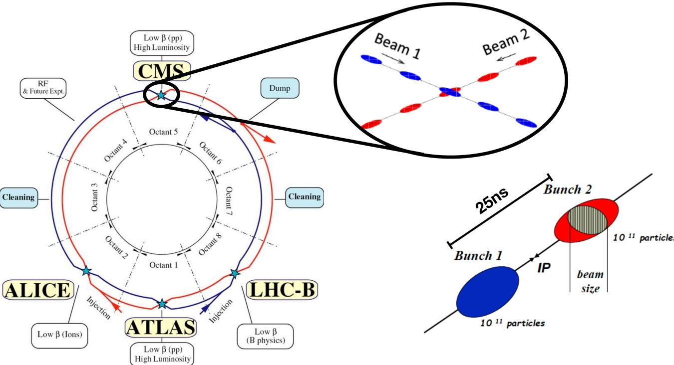
• The LHC accelerates *bunches of 10<sup>11</sup> protons* separated by 25ns gaps
