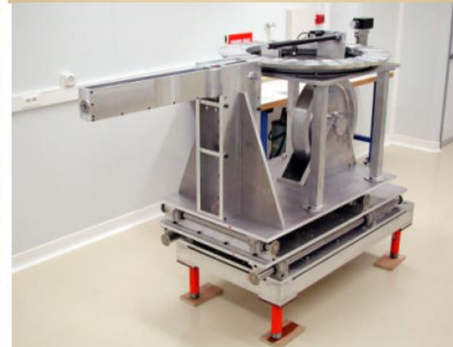
"Carousel" brick dispensing and storage system
