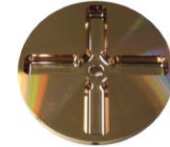
Accelerating structure prototype for CLIC: 12 GHz ( L \sim 25 cm)
