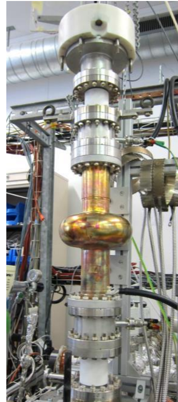
DC magnetron sputtering of 1.3 GHz cavities at CERN
