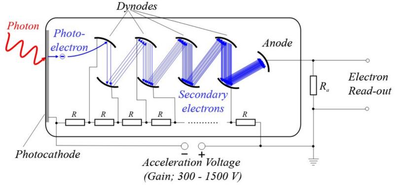
• High intrinsic gain (i.e.: amplification)  $\rightarrow$  no pre-amplifier required
