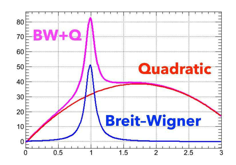
$$BW(x; D, \Gamma, M) \approx \frac{D\Gamma}{(x^2 - M^2)^2 + 0.25\Gamma^2}$$
