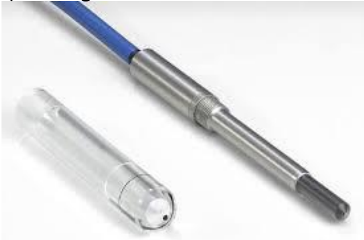
PTW TM30013 Farmer chamber (working horse for monitor calibration)
