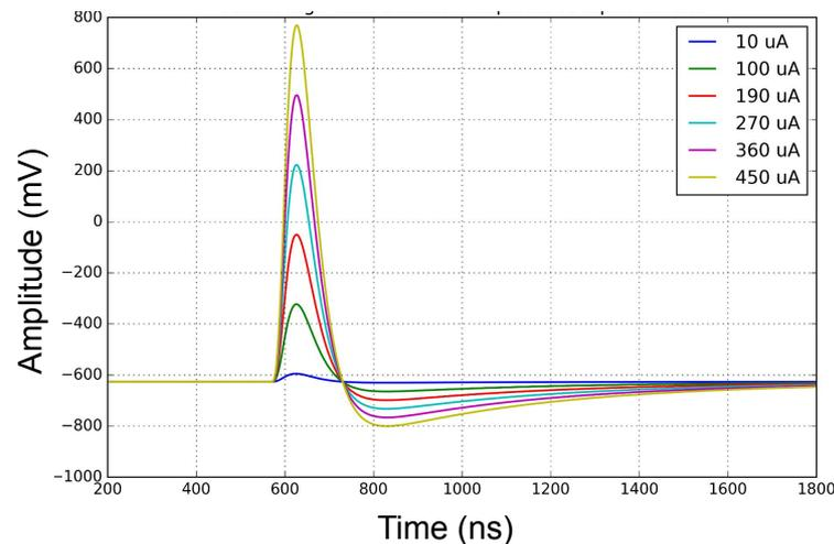
ALFE2 high gain output at different input signals. Phase has been interpolated 18 times.
