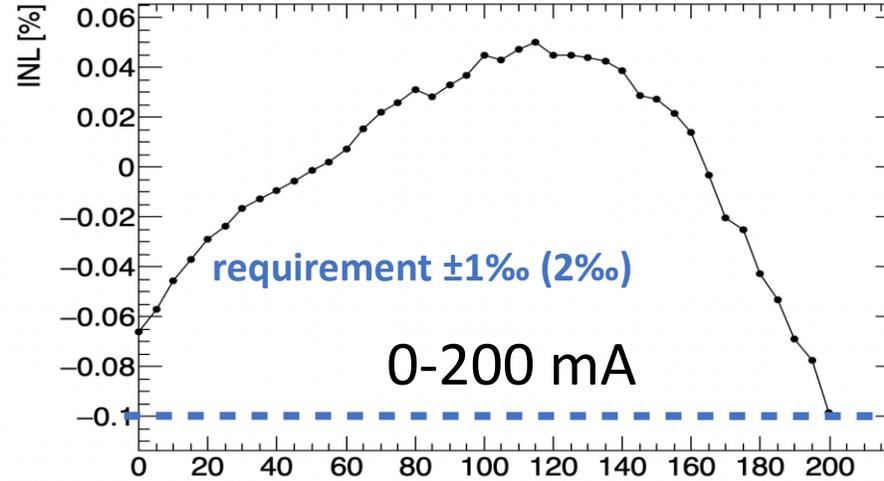
The INL is within specifications for small and medium ranges : output current < 200 mA
