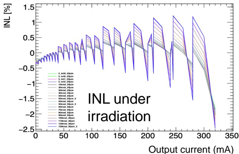
**Under irradiation (X-ray and protons)**
