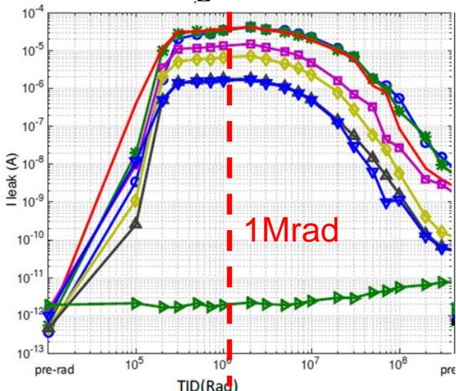
2.5V NMOS leakage current vs TID (From Michelis @CERN)
