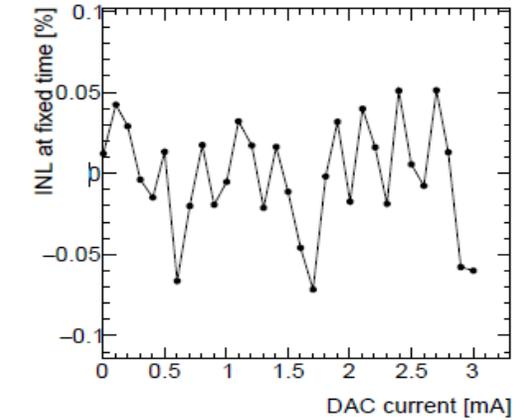
At low current, injected charge (pulse measured at DAC~0) has non-negligible effect on linearity
