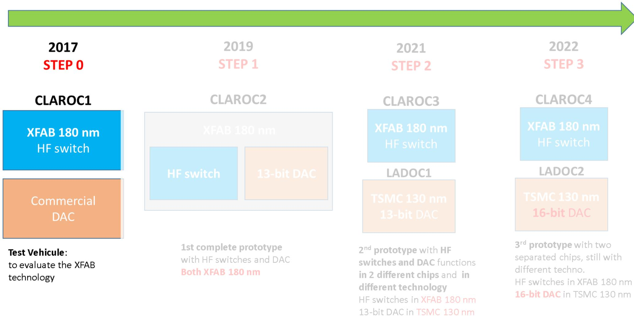
Chosen technology : **XFAB XT018** (180nm CMOS HV SOI)
