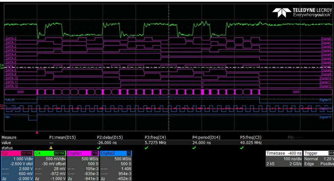
13-bit in parallel representing X,Y address of the touched readout-cell
