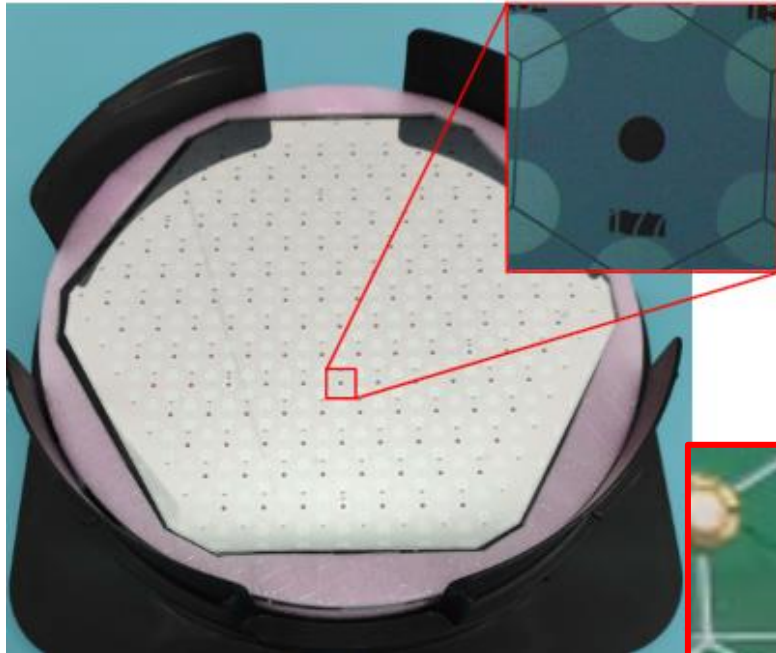
Silicon sensor with metallization opening(hole) in center of each cell, where laser can be injected
