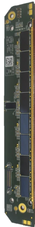
30 pcs of 2S front-end hybrids left (2S-FEH-L)
