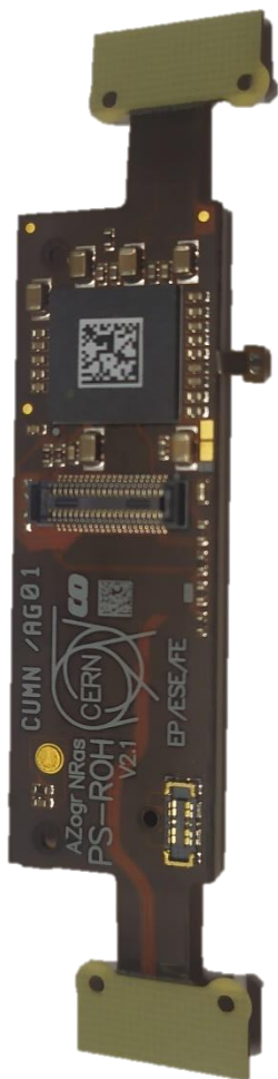
30 pcs of PS readout hybrid (PS-ROH)
