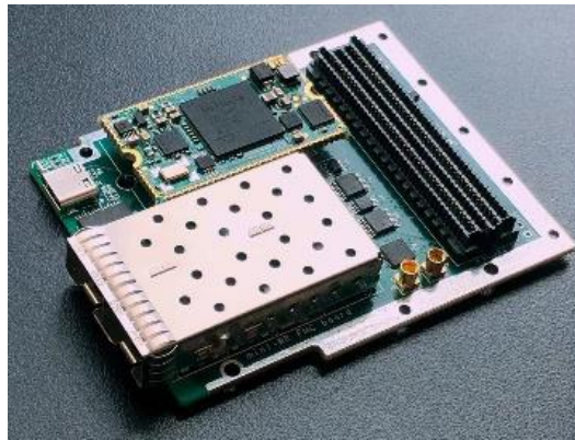
Mini-WR FMC for System-level clock synchronization
