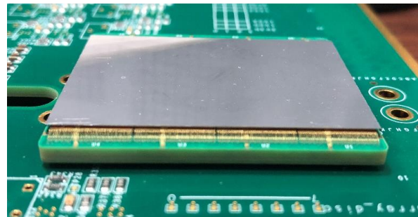
CuSn bump bonding module for the 2 nd prototype
