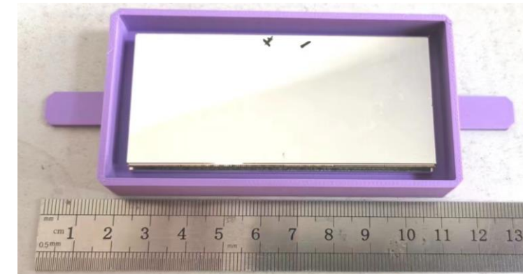
CuSn bump bonding module for the 4 th prototype after ASIC pin map optimization
