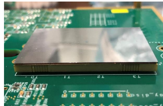
Bump bonding + TSV module for the 3 rd prototype
