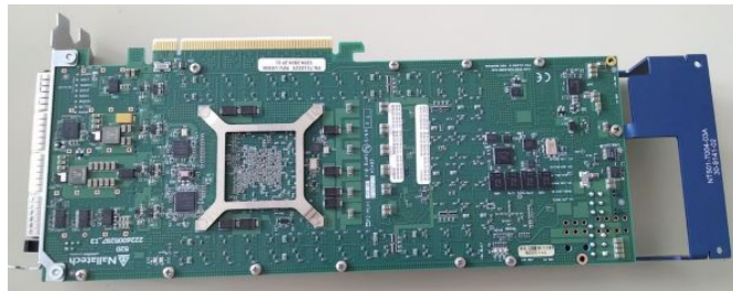
PCIe 16x board, 1 Intel Stratix 10 FPGA, 16 optical links
