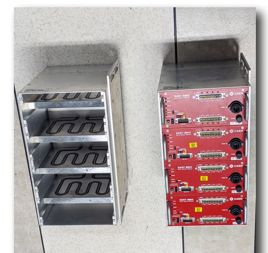
Figure 12: BRIC water cooled crate, on the left a detail of the inside with cooling pipe visible and on the right the crate mounted with all panels.
