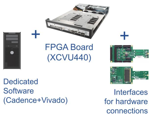
Dedicated Software (Cadence+Vivado) + FPGA Board (XCVU440) + Interfaces for hardware connections
