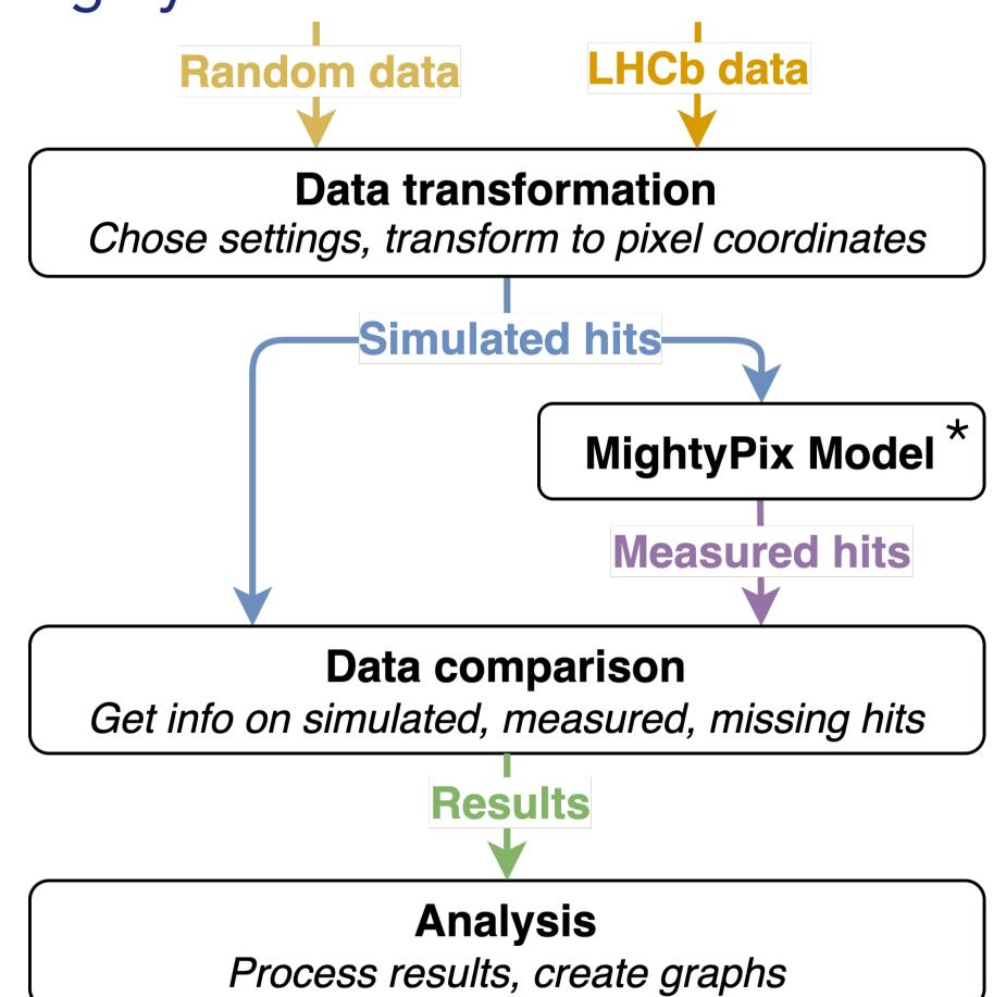
\* Behavioural model, representing analogue pixel matrix with synthesised digital logic
