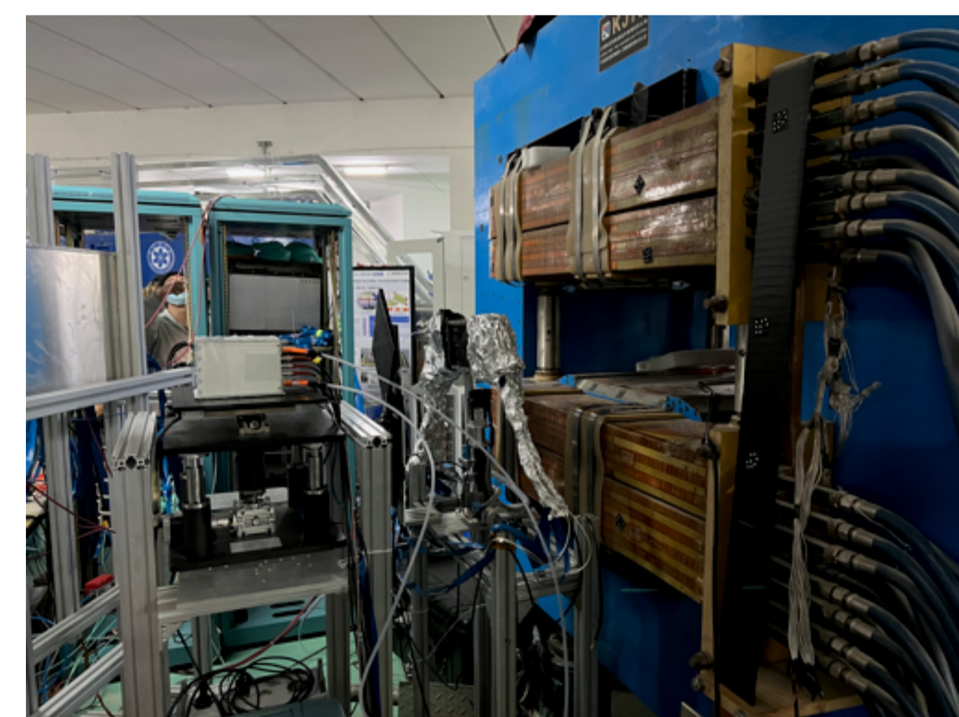
The setup of the beam test. The energy of the Fe-ion beam is 350 MeV/u, with the density varying between about 10^4 to 10^6 pps.
