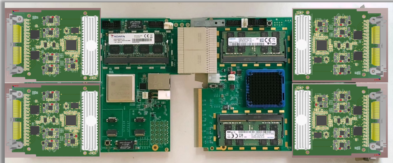
FEC BOARD (IHEP) max 128 channels
