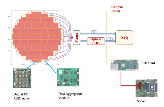
The readout plane consists of tens of modules, and the digitized pulses from all of the sensors will be transferred to the DAM modules on the edge. There will be around 20 high speed data transmission links between DAMs and the PCIe card in the DAQ system. The optical modules could be on the readout plane or on boards outside the TPC.
