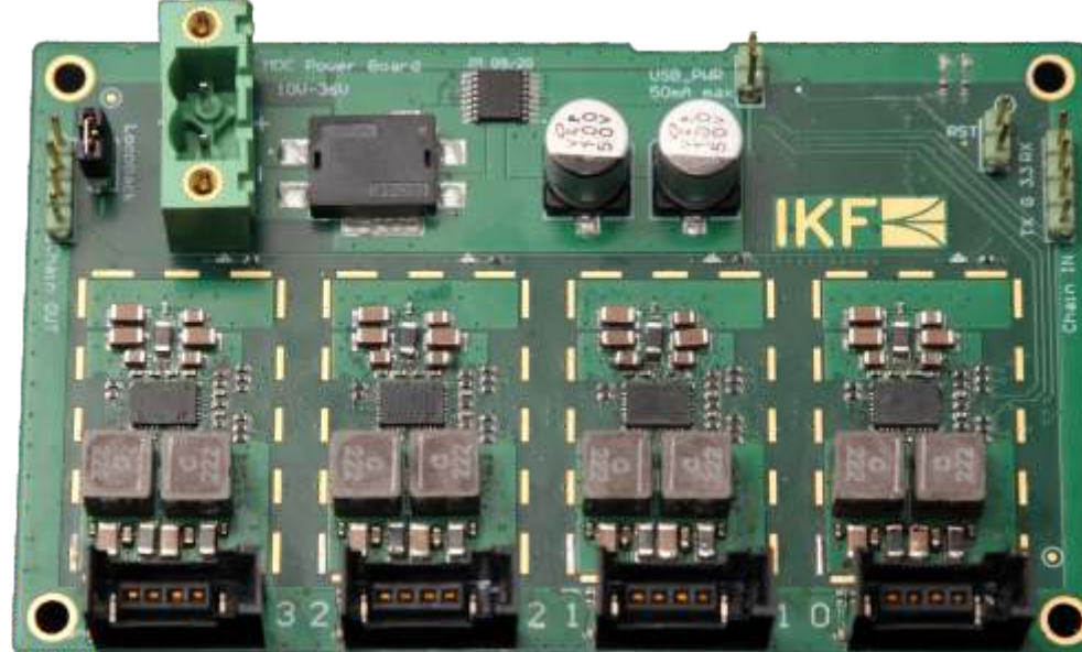
The voltage regulator board (4 channels) with adjustable low-noise DCDC converters
