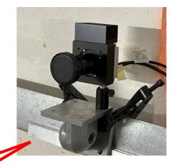
2x short exposure (1  $\mu$ s) cameras to cover 7 m of plasma for **space resolved** plasma light measurement
