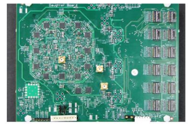
Figure 3. Circuit implementation. The left board realizes the analog mixing and filtering. A sign waveform alternating at 2 GHz is implemented in the right board.
