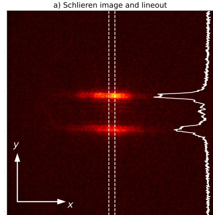
Laser probes changes in  $n(x,y,z)$  – vapor  $\leftrightarrow$  plasma
