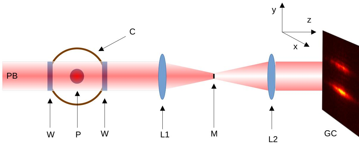
Laser probes changes in  $n(x,y,z)$  – vapor  $\leftrightarrow$  plasma
