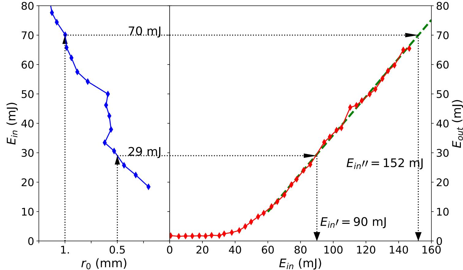
Compared experiment to simulated measurement → probe parameters are important!
