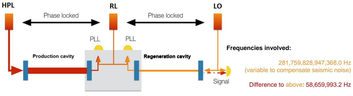
Down-mixing for signal detection:
