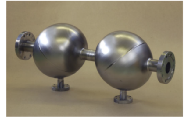
Figure 5. Niobium spherical cavities (fixed coupling).
