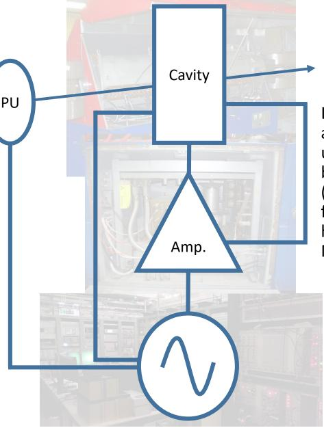
Local feedback systems around the cavity are used to reduce effects of beam induced voltage (e.g. one turn delay feedback 1TFB, multi harmonic feedback MHFB)
