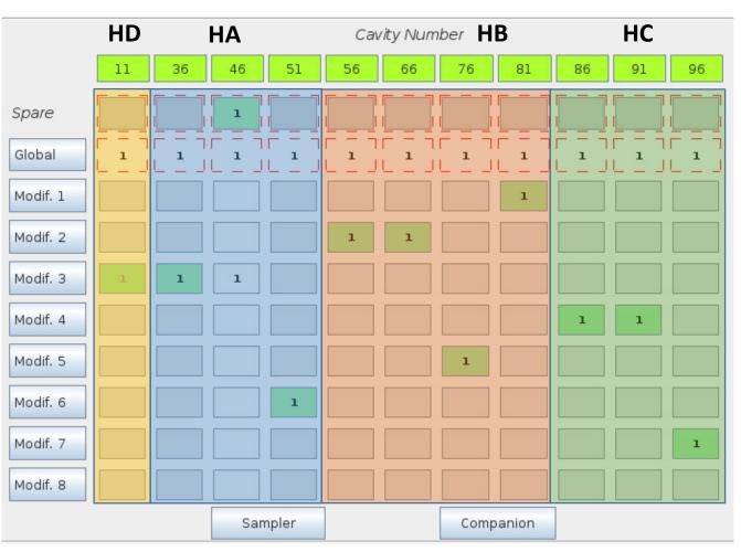
The voltage program for a cavity is the product of settings:  $V_{\text{cavity}} = V_{\text{global}} \times V_{\text{reduction}} \times V_{\text{modif}}$
