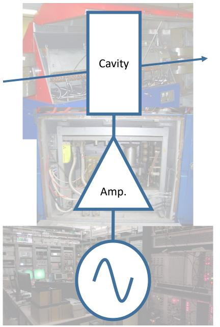
The power is transmitted in the RF gap where the beam passes and gets accelerated, manipulated, modulated...
