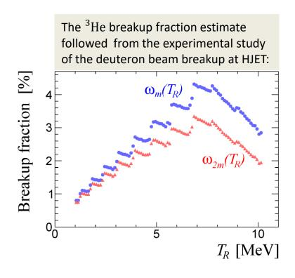
Effect of the helion breakup is negligible in the EIC <sup>3</sup>He beam polarization measurement using HJET.
