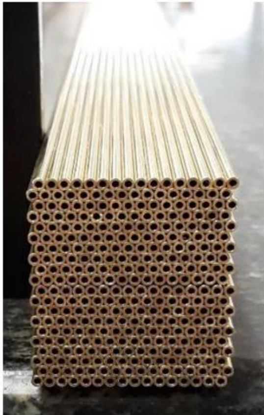
Copper rods outer diameter: 2.4 mm, inner diameter: 1.2 mm
