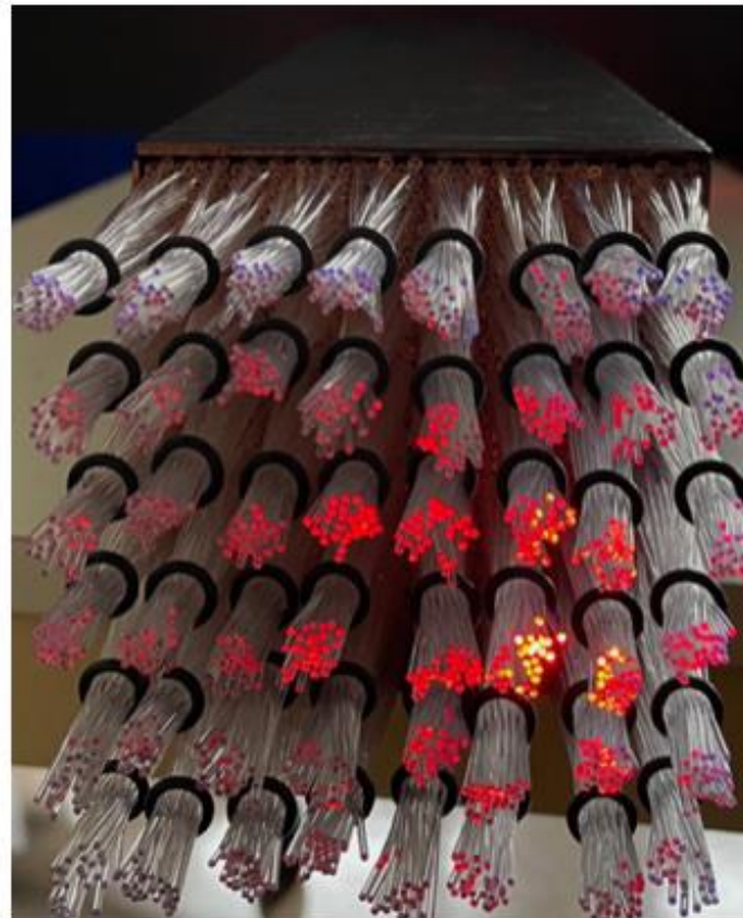
Prototype calorimeter tower 10x10x55 cm 3 built from copper rods equipped with scintillating fibers
